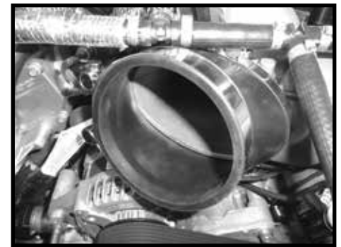
Step 16 Install intake manifold coupler and tighten one clamp.
