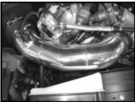
Step 19 Install intake tube, Align and tighten clamps. Install MAF sensor extension cable attach to factory wiring harness. Make sure it does not interfere with any moving parts.
