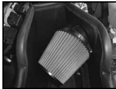
Step 15 Install air filter. Clock so filter has clearance on all sides.
