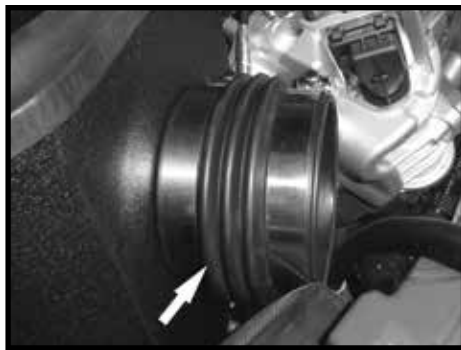
Step 14 Install flex coupler onto air filter velocity funnel and tighten one clamp. Note; push coupler on all the way making sure funnel is tight to heatshield.
